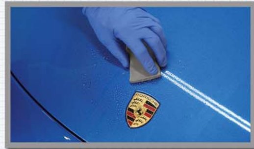
Clay bar cleaning.
